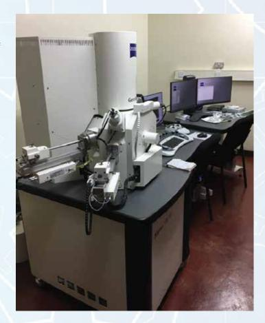
graphite derived nanomaterials will be determined by the purchased VP Sigma Scanning Electron Microscopy
