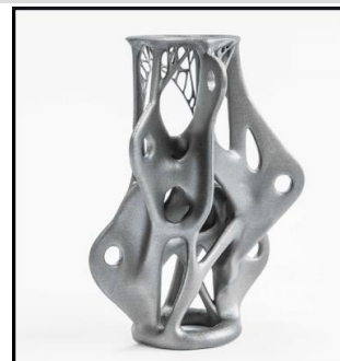
Complex shaped Additive Manufactured Part (Source: Yoders, 2014)
