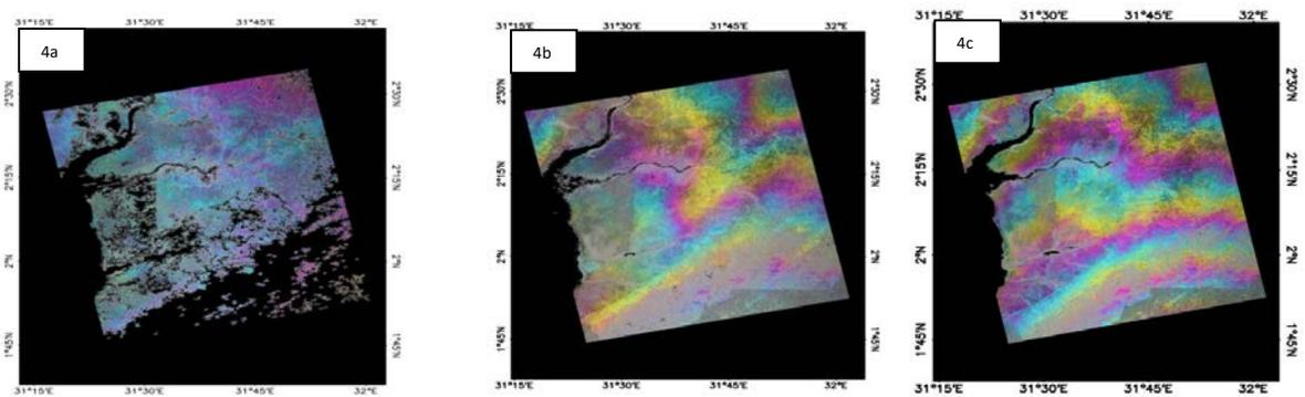
Figure 4: Differential interferograms
