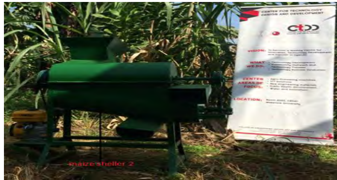
Improved maize sheller made at CTDD
