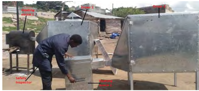
CTDD officer measuring temperature on heating source chamber
