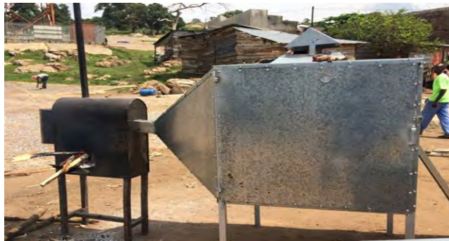
Hybrid dryer with heating source utilizing biomass
