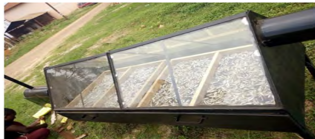
Hybrid fish dryer drying silver fish
