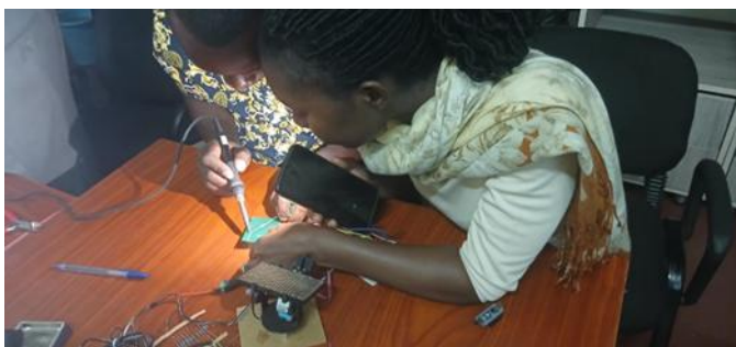
Figure 9: A team soldering the circuit board for the solar tracker
